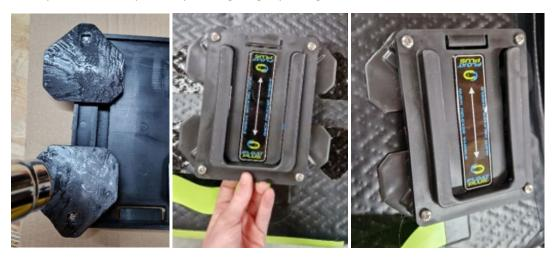
Carefully unscrew the sliders from the pads and press firmly, especially the edges. Keep checking and pressing on the pads and, if necessary, stick tightly with tape.
