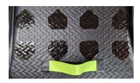
Apply the glue to the pads in the same way. Make sure the edges of the pads also have enough glue.
